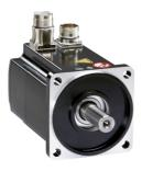
servo motor BMH, Lexium 32, 84Nm, 3800rpm, keyed shaft, with brake, IP54, 128bit encoder, straight
