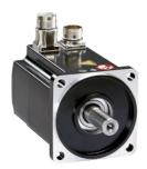
servo motor BMH, Lexium 32, 84Nm, 3800rpm, untapped shaft, with brake, IP65, IP67, 128bit encoder, straight
