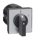
Cam switch, Harmony K, front mounting, plastic, 3 poles, 90°, 63A, 64x64mm, marked OFF/ON
