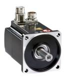
servo motor BMH, Lexium 32, 34.4Nm, 3800rpm, untapped shaft, with brake, IP54, 128bit encoder, straight
